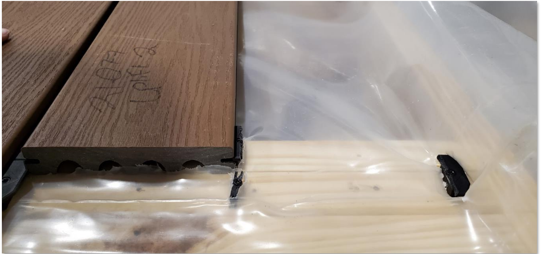
Photo 4. Predominant failure mode of the uplift resistance test.
