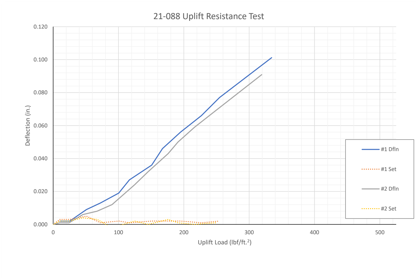
Figure 2. Deflection versus load plot of the uplift resistance test.
