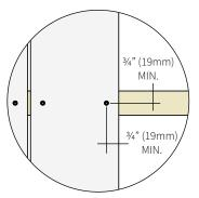
Screws should be a minimum of ¾" (19mm) from the board ends and edges.
