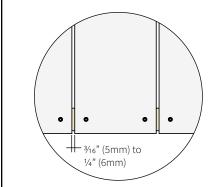
Allow 3/16" (5mm) to 1/4" (6mm) edge-to-edge spacing between deck boards.
