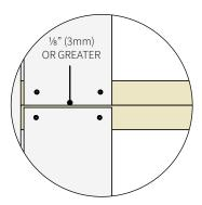
Allow 1/8" (3 mm) or greater end-to-end spacing between boards (butt joints).
