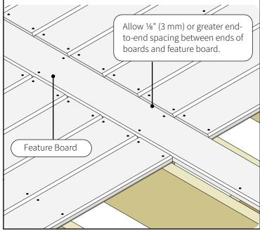
Pro Tip: Staggering the butt joint improves the overall appearance of the finish deck.
