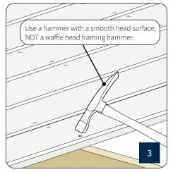
**Step 3:** Tap the material with a flat hammer to compress it into the hole. Vantage will self-heal with sun exposure.
