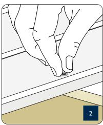
**Step 2:** Using your thumb, gently push the displaced decking material into the hole left by the screw.
