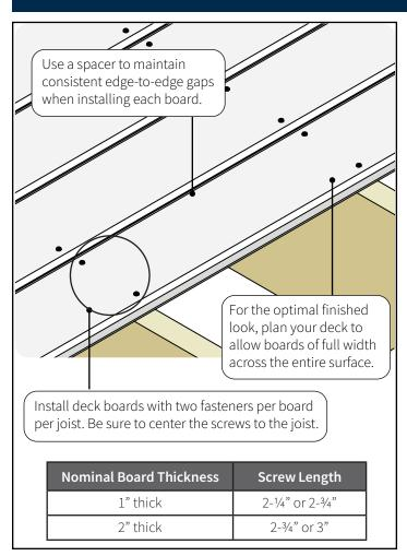
Pro Tip: Using a 2" (50.8 mm) driver bit allows you to better gauge screw depth. Once all boards are in place, snap a blue chalk line across the ends of the boards to the desired overhang. Leave at least 3/16" (5mm) overhang to conceal rim joist imperfections.
